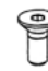
x 2 Round head screw E (0.197" x 0.63") Tornillo soporte red E M5x16 mm
